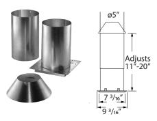
Required for installations that pass through an attic to prevent insulation from accumulating near the vent. Provides 1" clearance to combustibles.
